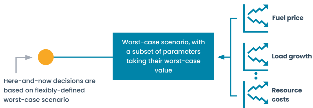
FIGURE 3. Illustrative schematic of robust optimization in the context of resource planning.
